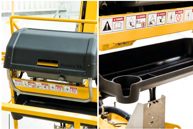
ULTRA-DURABLE PROTECTIVE HOUSING AND TOOL TRAY made of composite material
